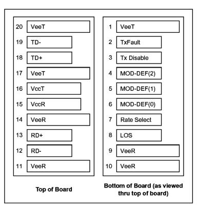
Pin out of Connector Block on Host Board
